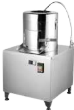
Potato Peeler SY8: 490×480×800mm, 8Ltrs., 240- 480Kg/hr SY15: 570×535×900mm, 15Ltrs., 480-900Kg/hr
