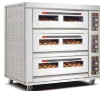
3 Deck 9 Tray, EBO 39 Dimension: 65.35 x 32.28 x 60.24 inches Chamber: 51.18 x 25.2 x 8.46 inches Power: 25.2Kw, 380v
